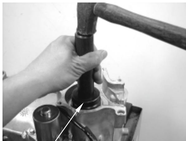
Oil Seal And Bearing Install
